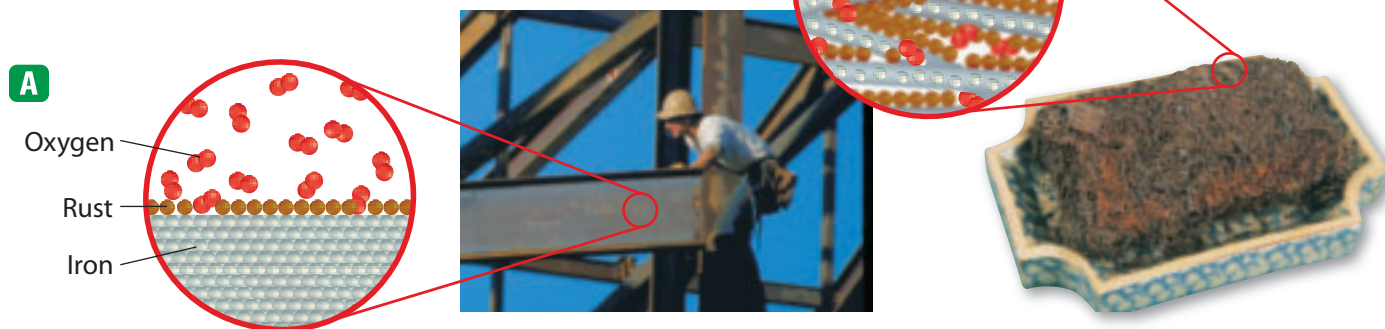
Figure 17 Iron atoms trapped inside this steel beam cannot react with oxygen quickly. More iron atoms are exposed to oxygen molecules in this steel wool, so the reaction speeds up.
