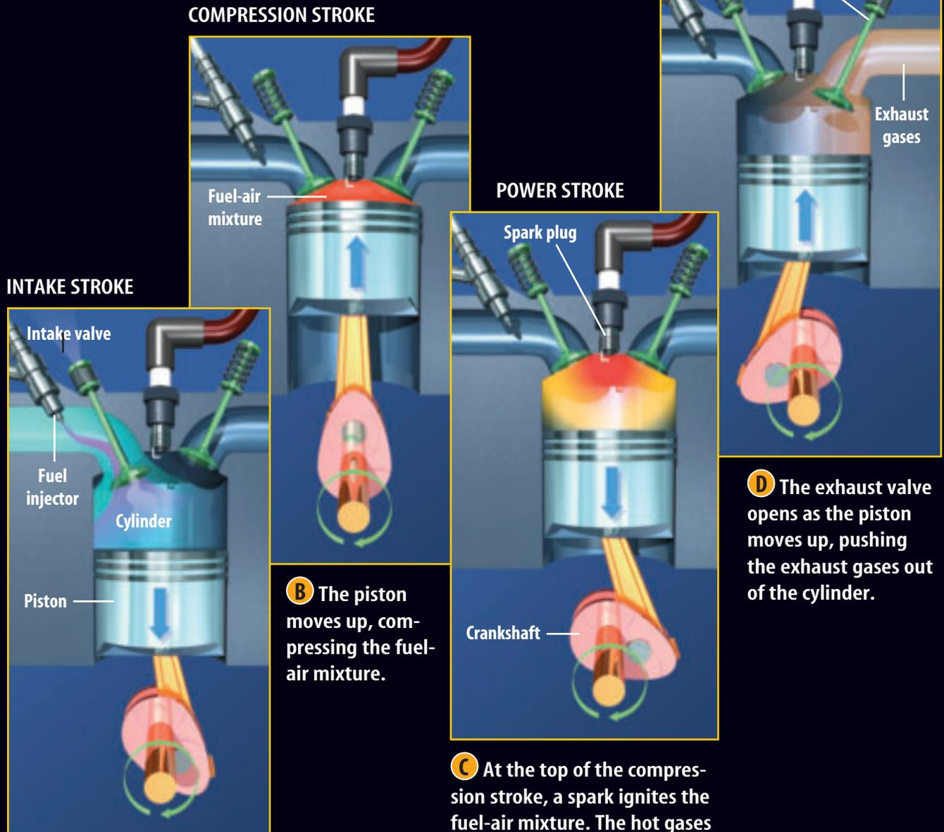
**A** During the intake stroke, the piston inside the cylinder moves downward. As it does, air fills the cylinder through the intake valve, and a mist of fuel is injected into the cylinder.
