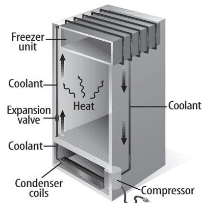
14. The illustration above shows the parts of a refrigerator and how coolant flows through the refrigerator. Explain how thermal energy is transferred to the coolant inside the refrigerator and then transferred from the coolant to the outside air.
