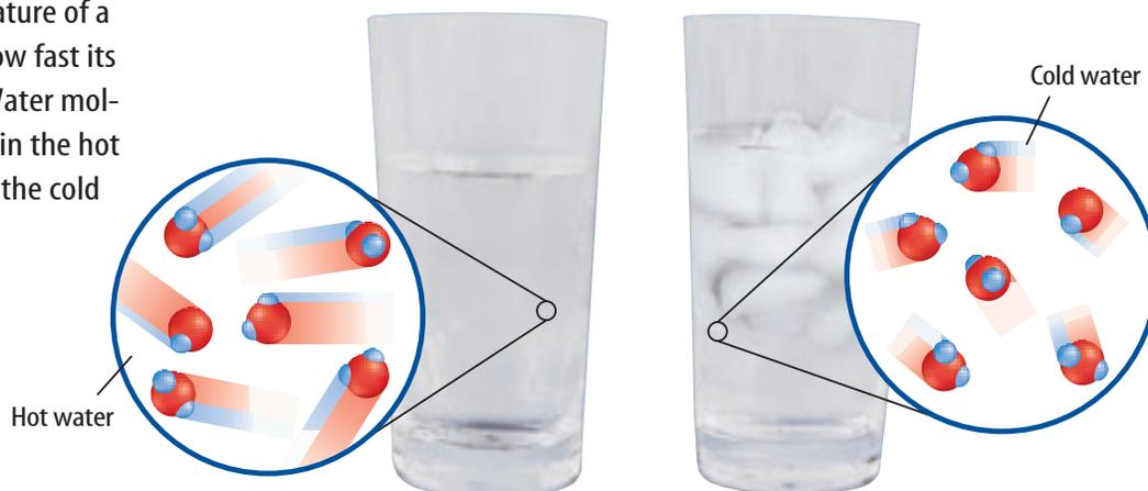
**Thermal Expansion** It wasn't an earthquake that caused the sidewalk to buckle in **Figure 2**. Hot weather caused the concrete to expand so much that it cracked, and the pieces squeezed each other upward. When the temperature of an object is increased, its molecules speed up and tend to move farther apart. This causes the object to expand. When the object is cooled, its molecules slow down and move closer together. This causes the object to shrink, or contract.
