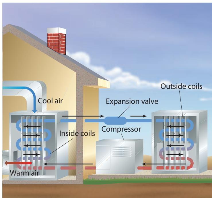
**Figure 15** A heat pump heats a building by absorbing thermal energy from the outside air and transferring thermal energy to the cooler air inside.
