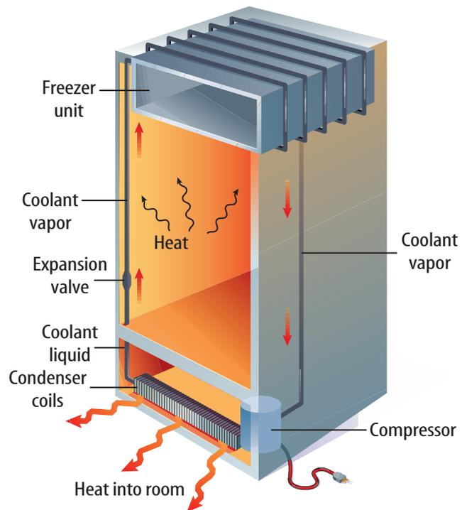
**Air Conditioners** Most air conditioners cool in the same way that a refrigerator does. You've probably seen air-conditioning units outside of many houses. As in a refrigerator, thermal energy from inside the house is absorbed by the coolant within pipes inside the air conditioner. The coolant then is compressed by a compressor, and becomes warmer. The warmed coolant travels through pipes that are exposed to the outside air. Here the thermal energy is transferred to the outside air.
